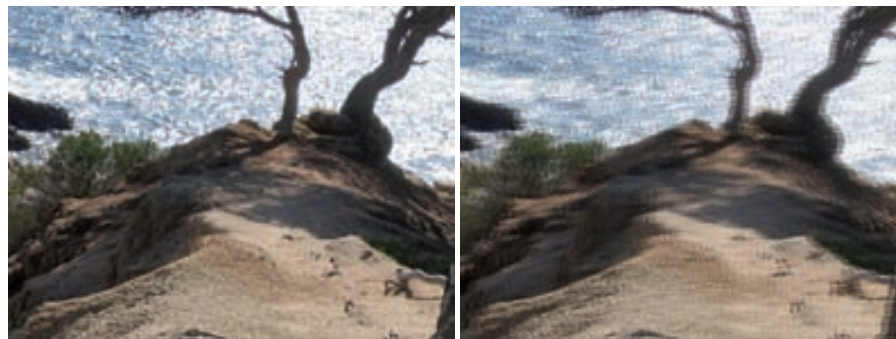
Figure 4.6: A progressive frame from a test sequence (left), and the same frame of the interlaced version of the video sequence (right).
