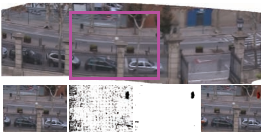
Figure 3.5: Example of an outdoor scene. The top image shows the background mosaic generated for this sequence. The bottom images show, from left to right: the original frame; the result obtained using a Gaussian background subtraction; the motion mask once we have applied the Markov Random Field background subtraction method proposed in the previous chapter; the motion mask overlapped with the frame.
