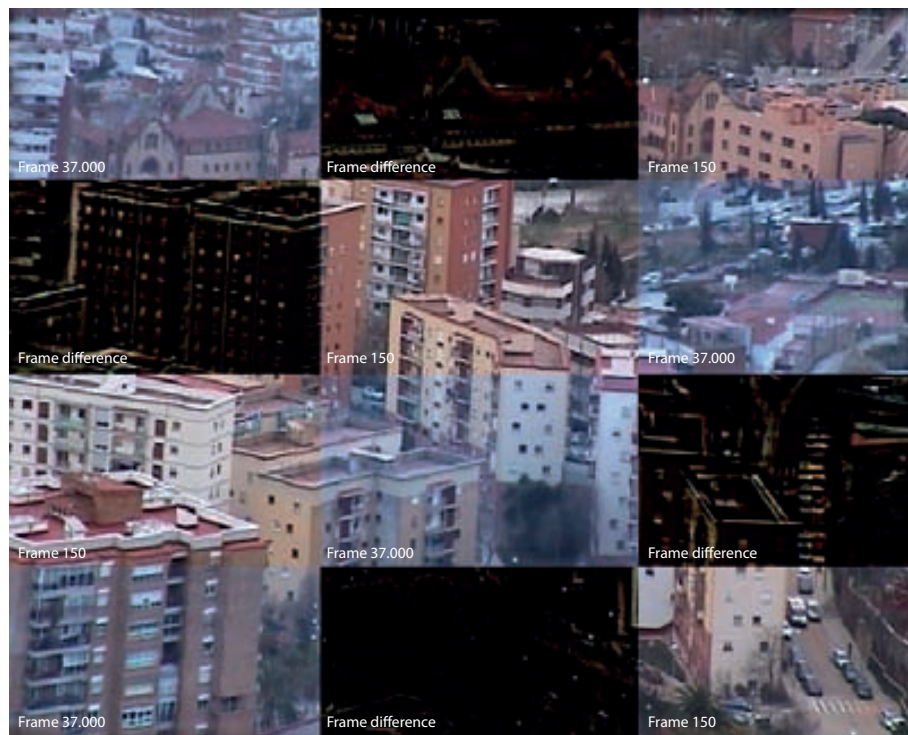
Figure 4.8: Comparison of light changes in a long interlaced sequence recorded using a Sony handycam DCR-PC110E. The blocks building the image correspond to frame 150, frame 37000, and their difference. It is important to note the color change, which produces some differences when subtracting the frames.
