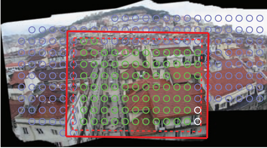
Figure 3.3: Example of target region configuration. The red box represents the area occupied by the current frame in the f_r space, the dashed box is the margin (only target regions that fit inside this box are selected), purple circles represent target regions of \mathbf{Q} that are not selected, green circles represent target regions selected to align the current frame (and they will be updated) and white circles represent target regions that added to \mathbf{Q} in this iteration.
