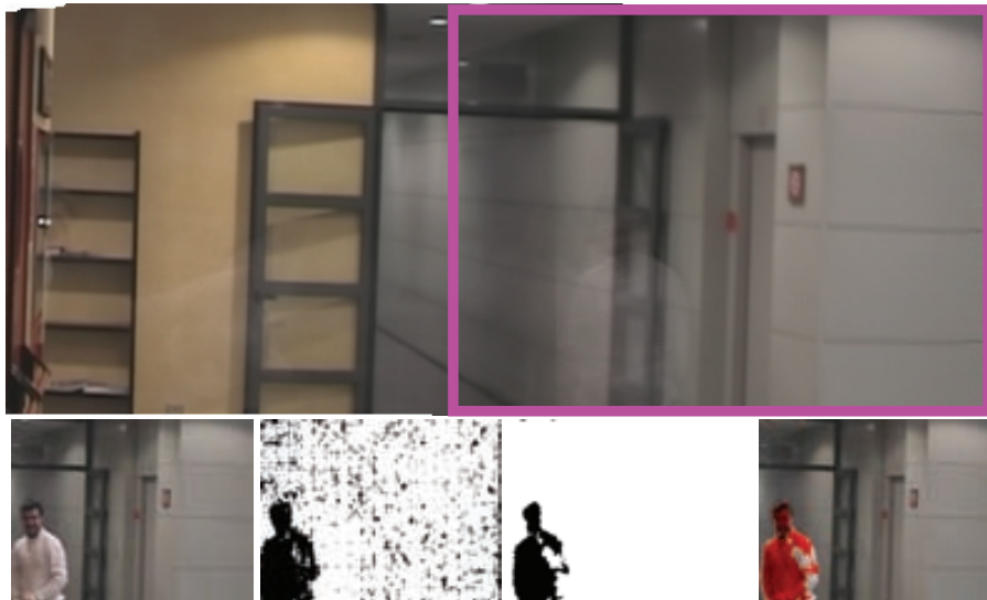
Figure 3.4: Example of an indoor scene. The top image shows the background mosaic generated for this sequence. The bottom images show, from left to right: the original frame; the result obtained using a Gaussian background subtraction; the motion mask once we have applied the Markov Random Field background subtraction method proposed in the previous chapter; and the motion mask overlapped with the frame.
