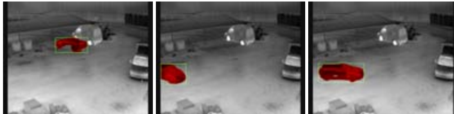
Figure 2.13: Motion segmentation using an IR sequence.
