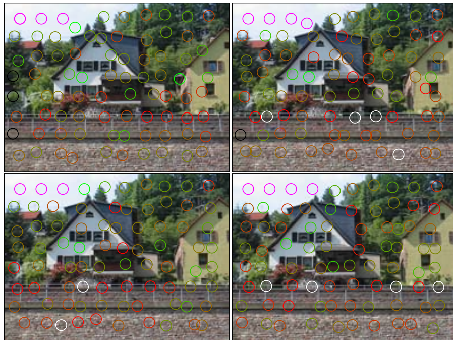
Figure 5.4: Evolution of some target regions in a video sequence. Each circle represents a target and the color its state. From green to red the SSD error (green less error) is represented. The targets detected on flat regions are pink, targets out of bounds are black and new targets white.
