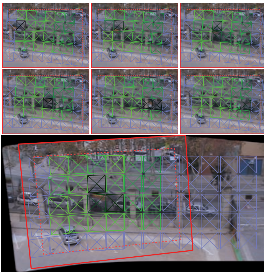
Figure 4.2: Green squares are patches centered at \hat{X}_i^j . The intensity of the color reflects the weights used by the WMSE. Those regions over the moving car have consistently low weight and therefore have a low impact on the alignment computation. The upper images are 4 consecutive frames; the lower image represents the corresponding mosaic.
