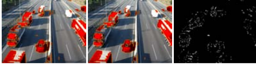
Figure 2.12: The left image shows the result of performing one iteration of BP. The center image shows the result of performing five iterations. The right image shows the difference between motion masks.
