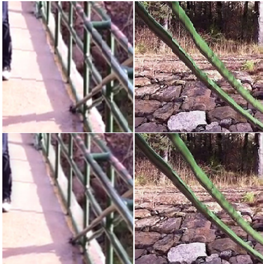
Figure 5.9: Comparison between mosaic regions with and without Barcode Blending. The top images belong to a mosaic image generated without any blending and the bottom images are generated using Barcode Blending.
