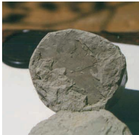
Fig. 6.14 Slickensides observed in a core recovered in borehole S1-3 at 13.5 m depth (Alonso & Gens, 2006a)
