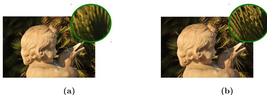
Figure 2.11: Effect of magnification change on feature shift (a) Focus at u = 4.6 m. (b) Focus at u = 8.7 m. Images captured with a Nikon D90 DSLR camera.
