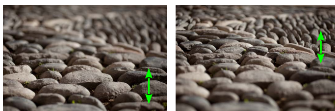
Figure 1.5: Effect of target position, u_x , on the depth-of-field. Left: target at u_x = 50 cm. Right: target at u_x = 70 cm. The depth-of-field increases when the camera focuses distant targets (right).
