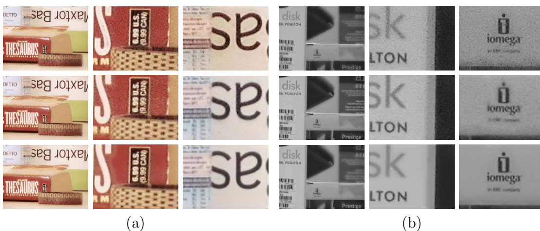
Figure 5.17: Image fusion for real focus sequences obtained with different algorithms. (a) For color focus sequence. (b) For gray-scale focus sequence. From top to down: first row, Helicon Focus software by Helicon Soft (2011); second row, 3D EDF algorithm (Aguet et al., 2008); third row, proposed SAF algorithm.
