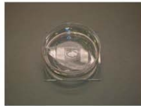
FIGURE 3: Assembly for a PoM device: The glass substrate with the ITO electrodes makes up the base. Mounted on top is a 35mm petri dish to hold the culture medium. A PDMS ring between glass substrate and petri dish seals the construct.
