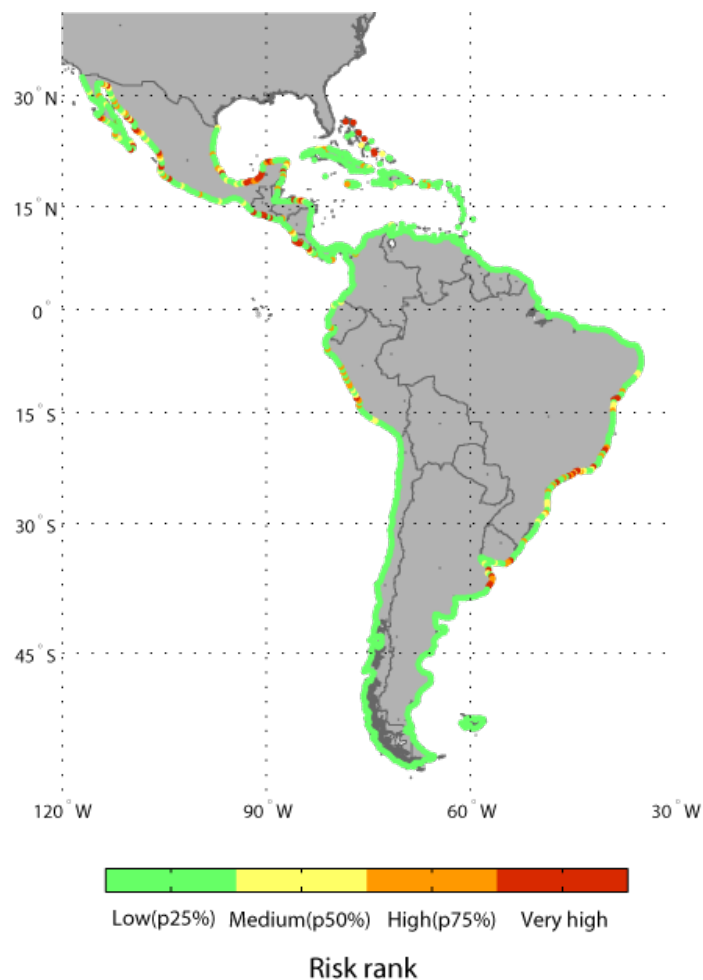
Figure 5.21: Risk levels for infrastructures (roads and rails) associated with 50-yr flooding event, by extrapolating to 2040 changes detected in the past extreme probability density functions.
