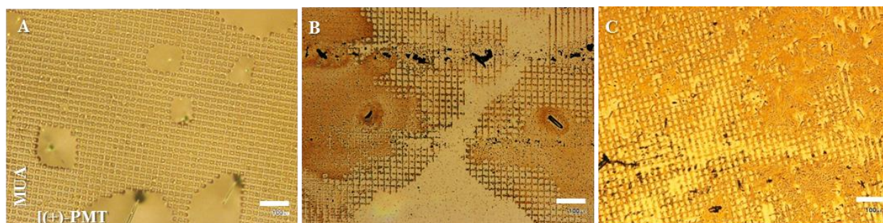
Figure 8.2.26. (-)-PMPP/ (-)-PEA salt crystallisation on micropatterned 10 x 20 \mu\text{m} lines with the cross printing surface method using (+)-PMT and MUA. Optical micrographs of: (A) after incubation time in crystallisation mushroom; (B) after drop drying; (C) after 5 days of incubation in (-)-PMPP/ (-)-PEA salt solution 25 mM; Scale bar 100 \mu\text{m} .
