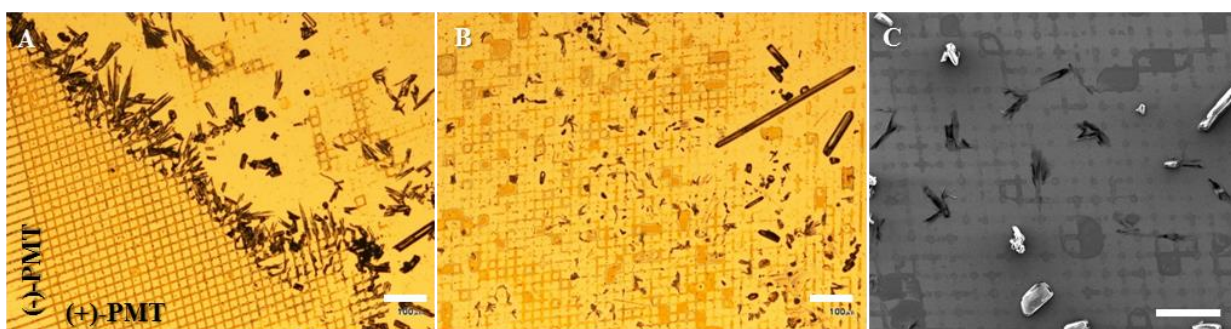
Figure 8.2.21. (-)-PMPP/(-)-PEA salt crystallisation on lines 5 x 10 \mu\text{m} micropatterned surfaces by cross printing surface: (A) After incubation time, (B) After washing with ethanol, (C) SEM micrograph of (B). The scale bar is 100 \mu\text{m} in all images.
