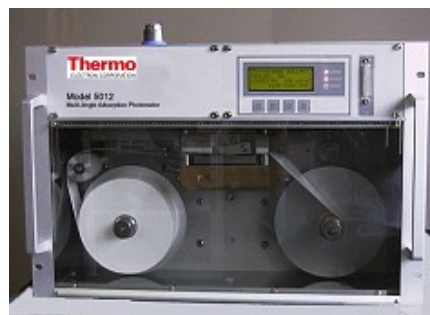
Figure 2.4. MAAP for BC measurements
