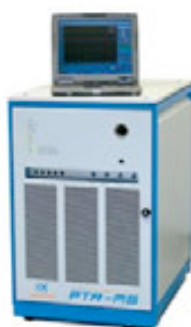
Figure 2.9. PTR-MS for on-line measurements of VOCs.
