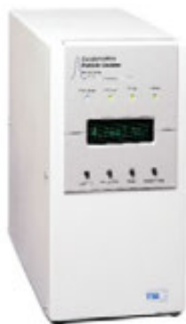
Figure 2.5. WPCPC TSI 3785 for measurements of number particle concentrations.
