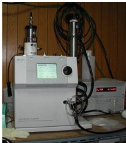
Figure 2.7. SMPS for measuring on-line segregated number aerosol concentrations.
