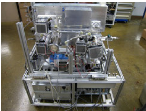
Figure 2.6. HR-ToF-AMS for online speciation of the non refractory fraction of PM.
