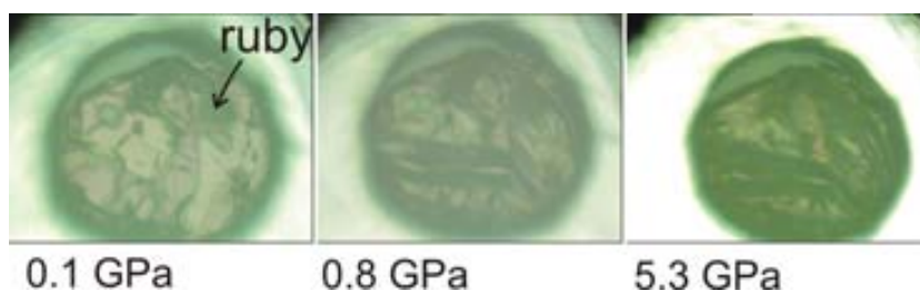
Figure 5.6: Photographs of a P3HT sample in the pressure cell taken in reflection.
