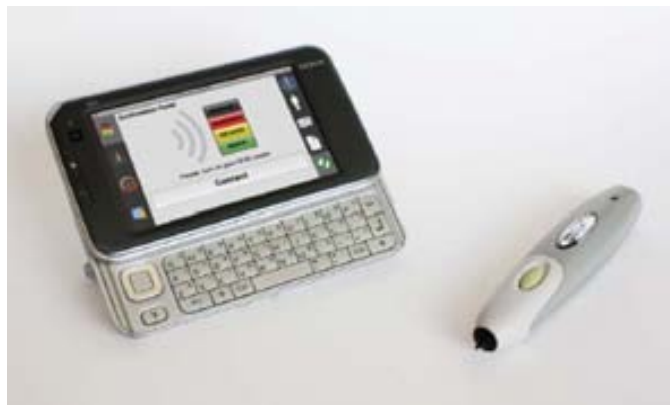
Fig. 3. Nokia N810 handheld device and ID Blue RFID reader components used in the implementation of MAETTS.
