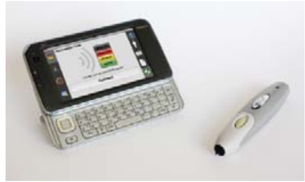
Figure 2: Nokia MAEMO n810 and RFID reader
