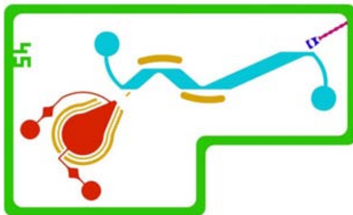
Figure 1. Design of the mask employed to fabricate the presented PhLoC. In red: emitter microstructure; in orange: air mirrors; in cyan MIR optofluidic system; in dark blue: microlenses; and in violet: self-alignment microchannel.
