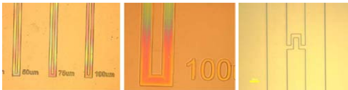
Figure 4. Optical images of waveguides of different widths. The light dark area at one side of each waveguide is the defined grating. Also, the sensing area of the 75 \mu\text{m} -wide waveguide is shown.
