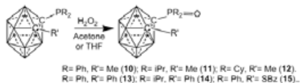
Scheme 2.1. Reaction of carboranylmonophosphines with hydrogen peroxide.
