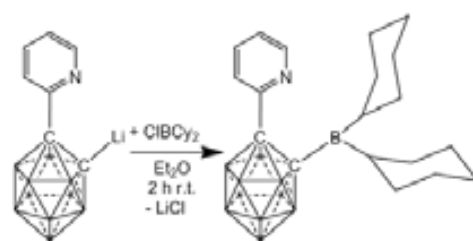
Scheme 4.8. Synthesis of carboranylpyridine-borane compound.
