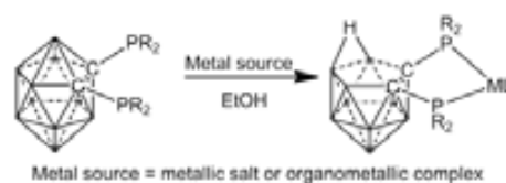
Scheme 2.10. Synthesis of organometallic complexes of nido -carboranylphosphines from closo -carboranylphosphines.
