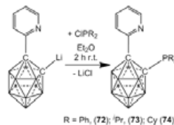
Scheme 4.5. Synthesis of carboranylpyridine-phosphine hybrid ligands.
