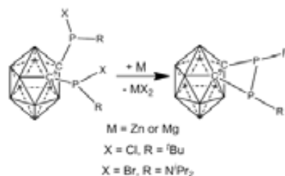
Scheme 2.2. Synthesis of carborane based 1,2-diphosphethanes.
