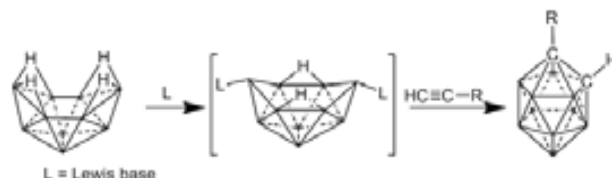
Scheme 4.1. General reaction scheme for the synthesis of carboranes from decaborane.
