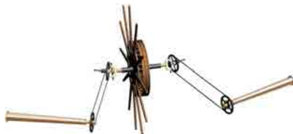
Fig. 10. Synchronism of the system. Application of gimbal joints to maintain the synchronism of the system, with a central winch.
