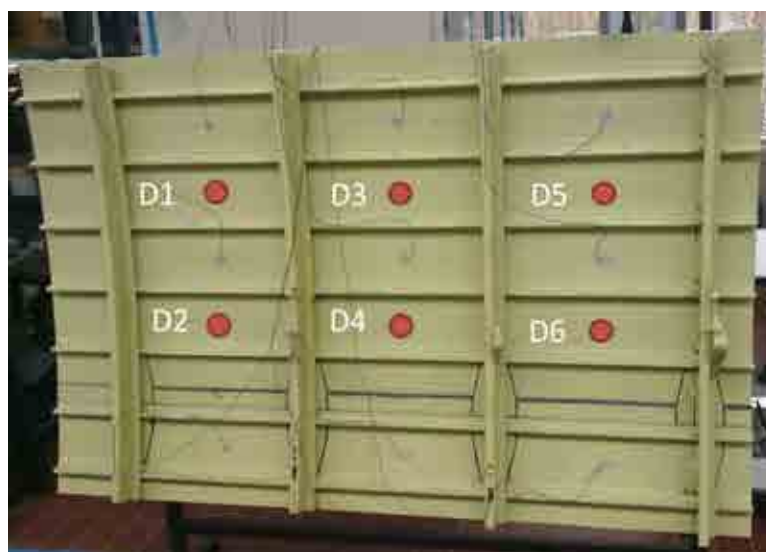
Figure 4.13: Damage distribution in the Airbus A320 Fuselage.
