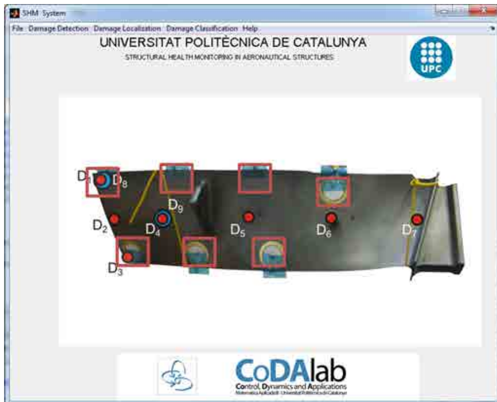
Figure 6.14: Interface for damage localization.
