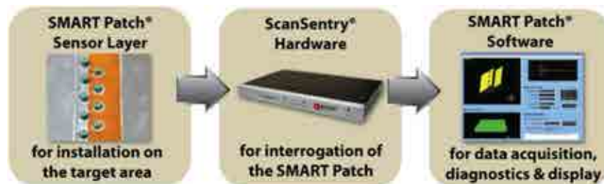
Figure B.5: Hot-Spot Monitoring [3].
