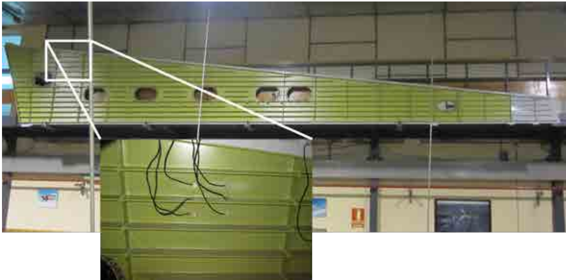
Figure 4.10: Sections tested with the PZT location.
