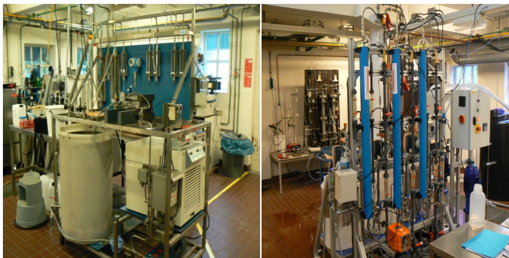
Figure 7.3: Images for the experimental set-up used in KWR a) flat-sheet using SEPA CFII (GE-Osmonics) cell; b) bench-scale for spiral wound membranes
