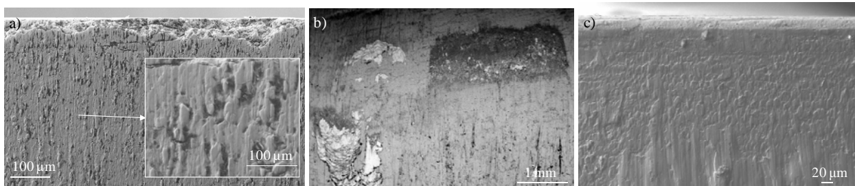
Figure 3.3.5 Wear related phenomena in tools: a) abrasive wear; b) adhesive wear; c) severe wear (abrasive + adhesive)
