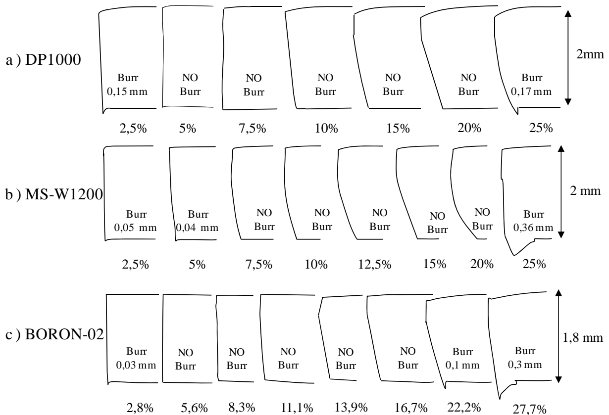
Figure 3.3.90 Schema of the punched sheet edge morphology of: a) DP1000 2 mm thick; b) MS-W1200 2 mm thick and c) BORON-02 1,8 mm thick for clearances between 2,5 % and 27,7 %
