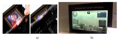
Fig. 1.5. a) SONY's organic thin film transistor driven, full color, flexible OLED display (80 µm-thick and 4 inches wide), able to reproduce moving images while being rolled around a cylinder with a radius of 4 mm., b) SAMSUNG's transparent smart window.
