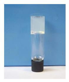
Fig 5.3.8. Self-supporting hydrogel of peptide (2-Thi)(2-Thi)VLKAA (2% wt in D<sub>2</sub>O).
