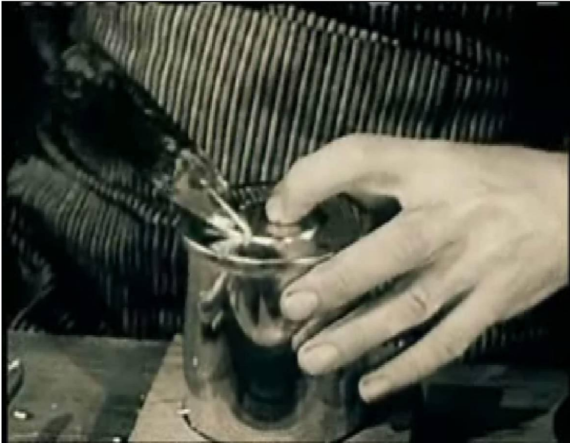
Figure 2.9. Worker welding the lid and the can by hand.
