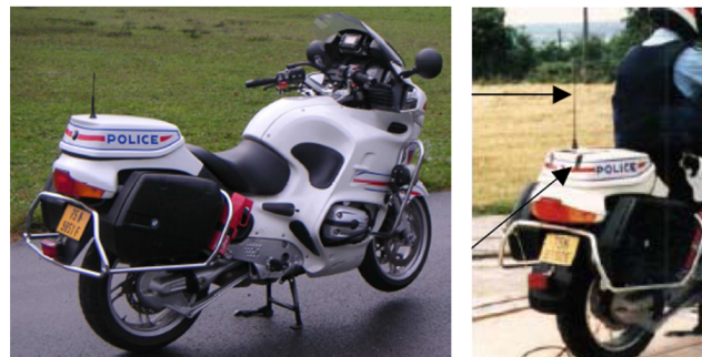
Figure 4.4: PROCOM MU9-XP4 antenna installed on a motorbike.
