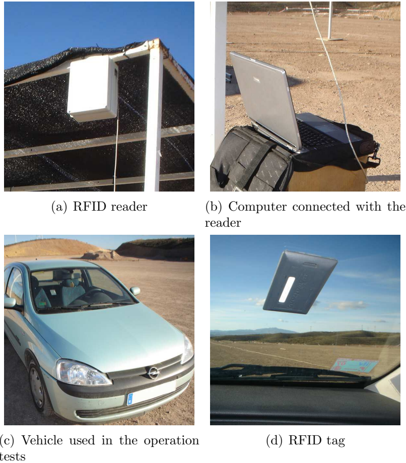
Figure 0.19: Hardware set-up of the RFID identification prototype
