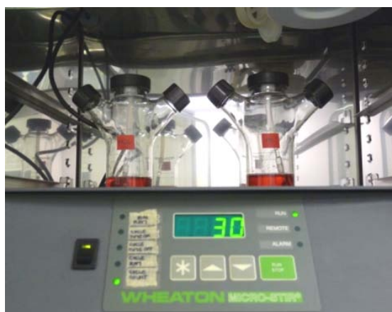
Figure 7.1. Spinner flask and rotating system used for the dynamic culture. The whole system was placed inside the incubator for the period of time the culture lasted.
