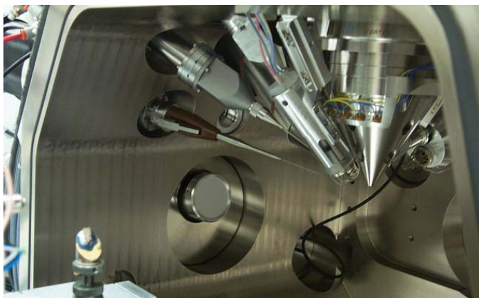
Fig. 3.10. Image of the chamber of the FIB equipment, with the different detectors employed to perform the different trenches 27 .
