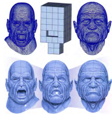
Figure 4.8: (Top) Sketching relevant features of two input models to be mapped on shared polycube domain allows to perform shape blending operations to create new models with shape details from the two (Bottom).
