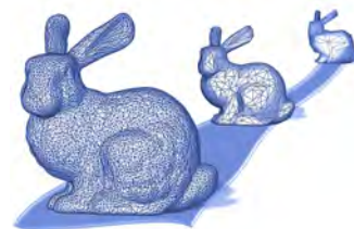
Figure 1.3: Level-of-detail techniques use simplified objects representations across the view distance.
