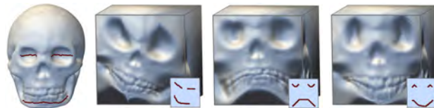
Figure 4.11: The users can take full control of the polycube map by simple sketches. The thumbnails show the sketched constraints.
