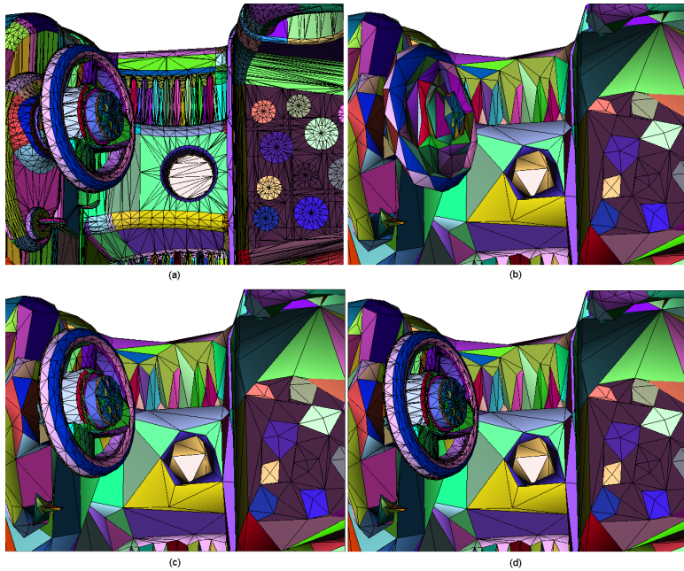
Figure 3.14: Original toy car model (a), model simplification to 10% (b) and refinements of the subobjects that make up the steering wheel at 50% (c) and 100% (d)
