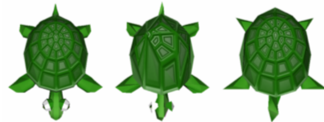
Figure 4.19: Front of turtle model. Original model (left) and the model simplified at 25% without applying our texture-based error metric (centre) and applying it (right)
