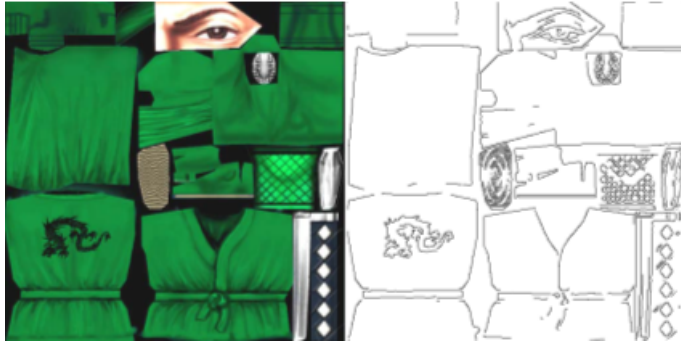
Figure 4.10: Borders of the ninja model detected by the border detection method with \sigma = 0.75 , low threshold = 0.5 and high threshold = 0.6
