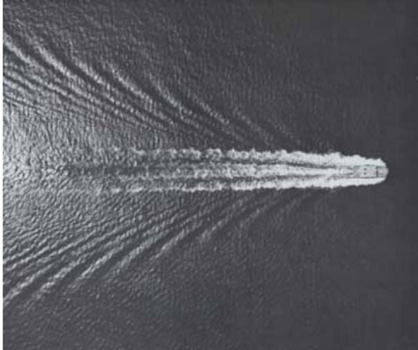
Figure 2.8: Kelvin wedge: V-shaped waves following a ship in movement (image captured from Google Earth).
