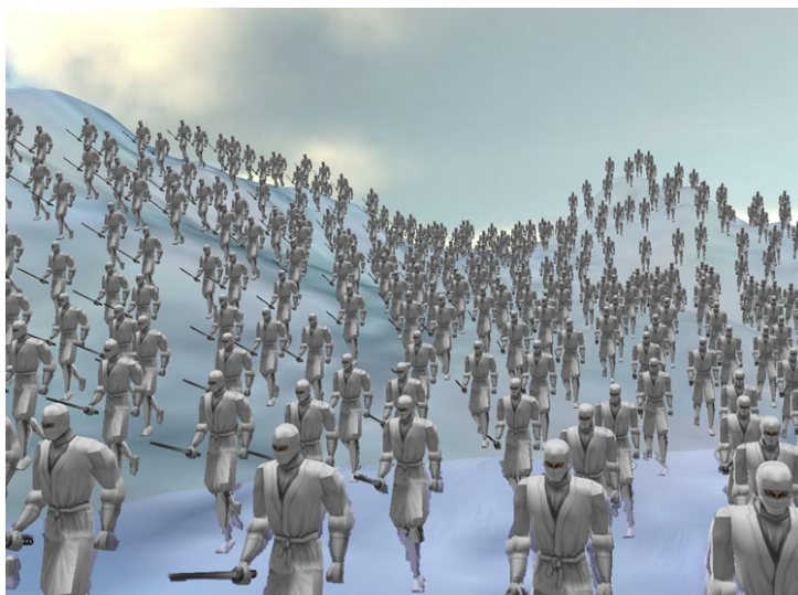
Figure 1.2: Continuous multiresolution models rendered at different levels of detail. According to the distance to the viewer, closer objects are more detailed and further less detailed.
