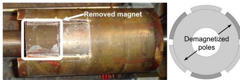
Fig.4.10. Rotor of the analyzed partially demagnetized SPMSM. It has 6 rows with 4 magnets/row
