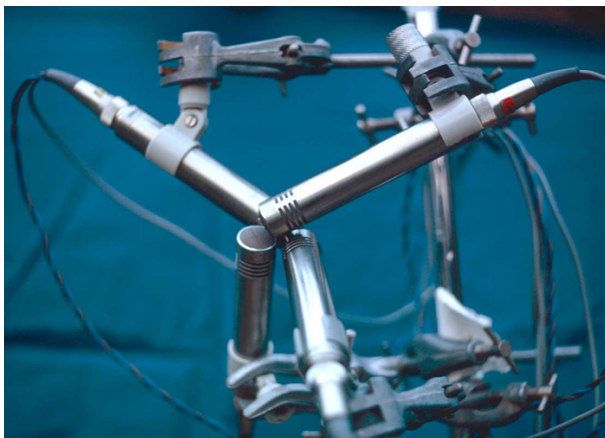
Figure 3.8: Four directional microphones in a tetrahedral arrangement for early Ambisonics recordings. Picture from http://www.michaelgerzonphotos.org.uk/tetrahedral-recording-images.html
