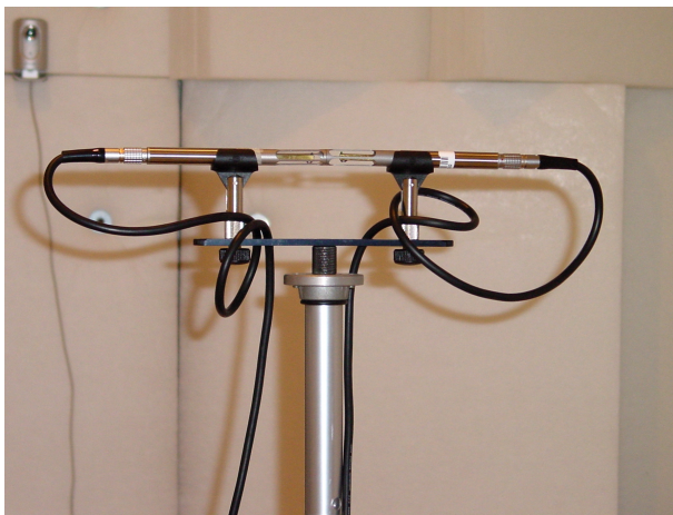
Figure 3.22: Two USP probes in face-to-face configuration. Protective caps limit minimum spacing to 20 mm, although they can be removed, allowing for a closer proximity.
