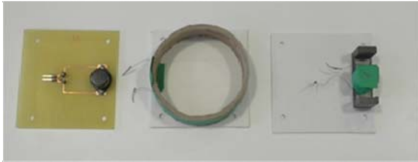
Fig. 5.3 Three different coil types. From left to right: Fastron commercial coil, air-core coil, ETD ferrite-core coil.
