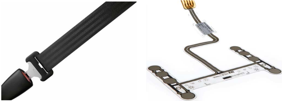
Fig. 1.1 Pictures of the belt (left) and seat occupancy (right) detectors employed in this thesis. Figures respectively taken from [14] and [15].
