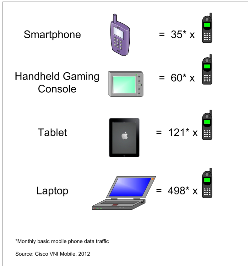
Figure 1.2: Traffic correspondence between high-end devices and conventional mobile phones
