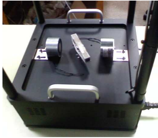
Fig. 6.2 Picture of the main part of the Roto-magnet plant: DC motor, optical encoder, magnetic system (load), and supporting structure.
