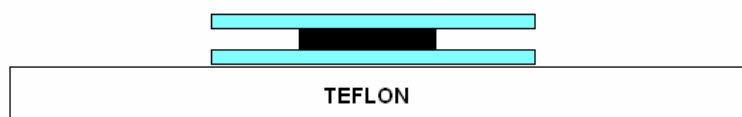
Figure 4.22. Glass press designed to reduce the contact between O_2 and the rubber surface.
