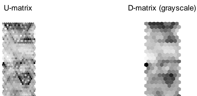
Figure 3.13. Visualization of the clustering structure of the SOM from the U-matrix (left) and the mean distance matrix (right) points of view. High distances are represented by dark gray colors, while lighter colors correspond to smaller distances
