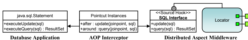
Figure 3.3: Example of Source Hook for JDBC.
