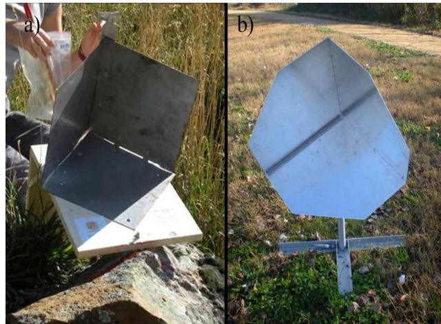
Figure 5.10: Two types of CRs developed and tested at the Institute of Geomatics.
