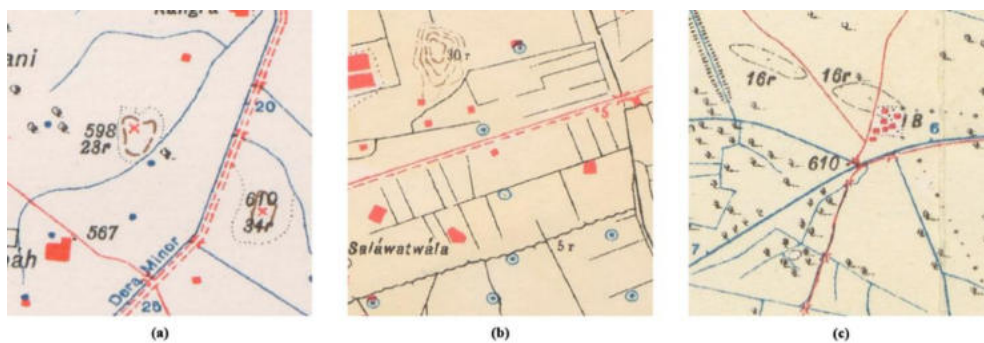
Figure 34. Different form-line typologies found in historical SoI maps: (a) dashed [23r] and solid line [34r] mound feature, (b) mound feature with concentric lines [30r], and (c) road-like black line mound feature [16r].
