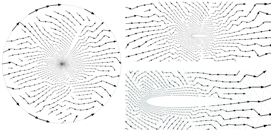
Figure 6.3: NACA0012: Node to node vectors forming the streamline linelets.
