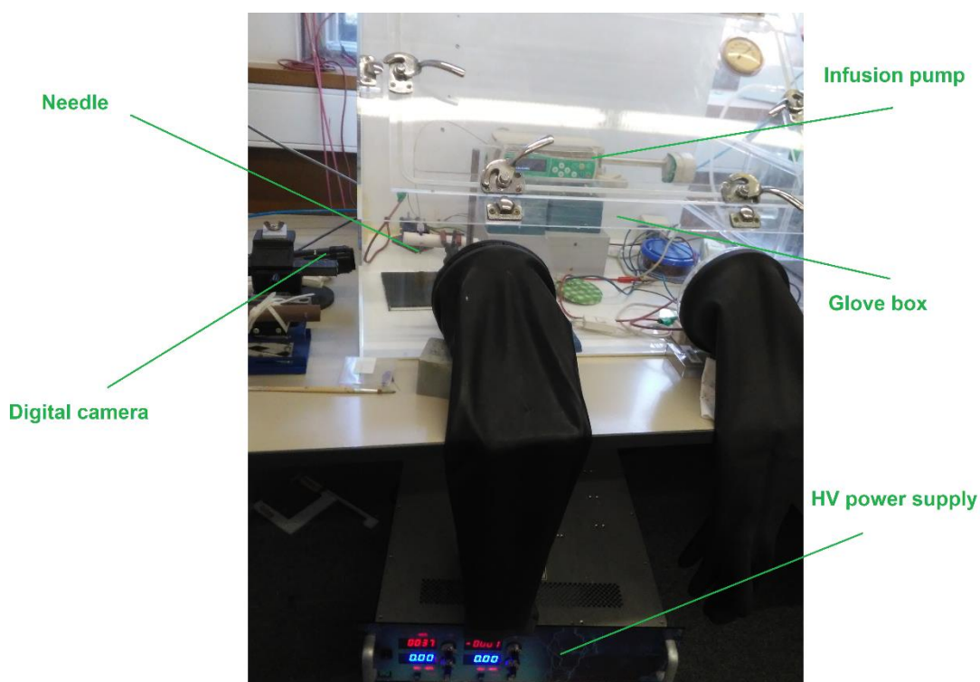
Figure 37. Electrospray system mounted in the UPC facilities.
