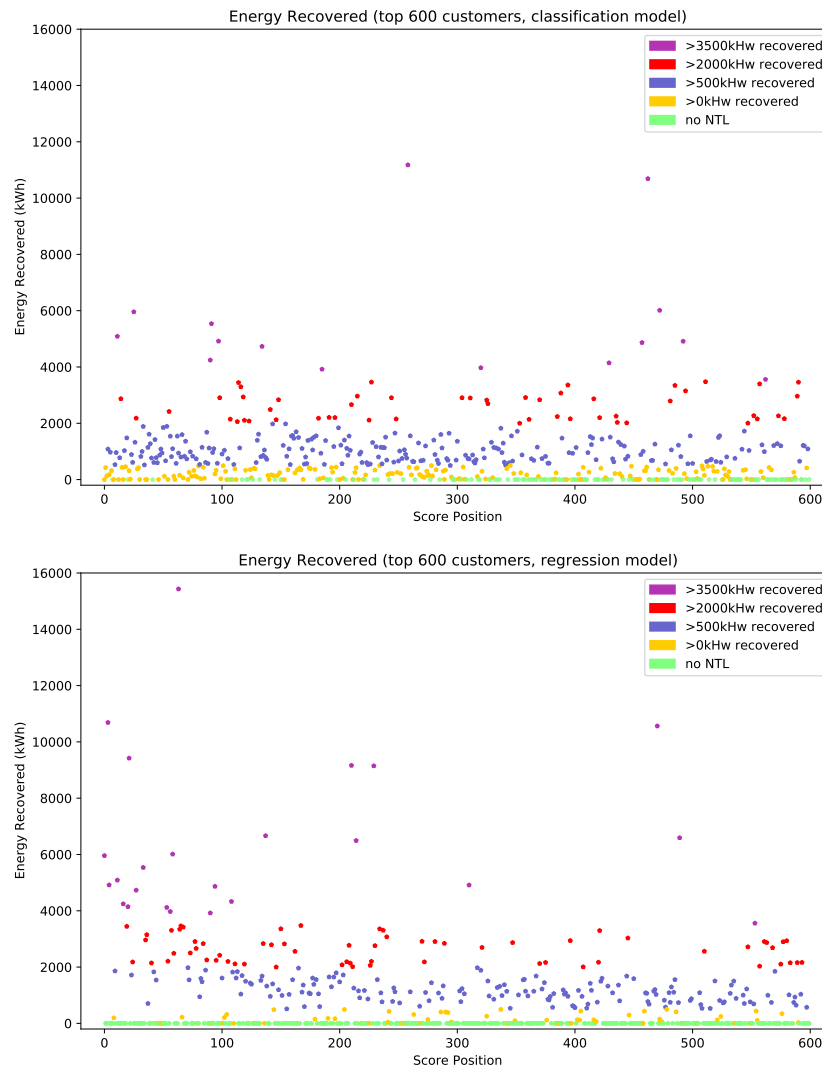
Figure 4.3: The results obtained in Table 4.1 are confirmed in these images: the regression model recovers more energy at the very top of the test prediction list. More specifically, we can see how the purple cases (NTL cases with more than 3500kWh, the average customer’s energy consumption per year) in the regression model are recovered at the very top of the rank.
