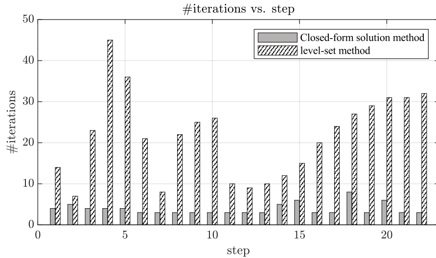
(b) Variational closed-form method vs. level-set method: computational cost
