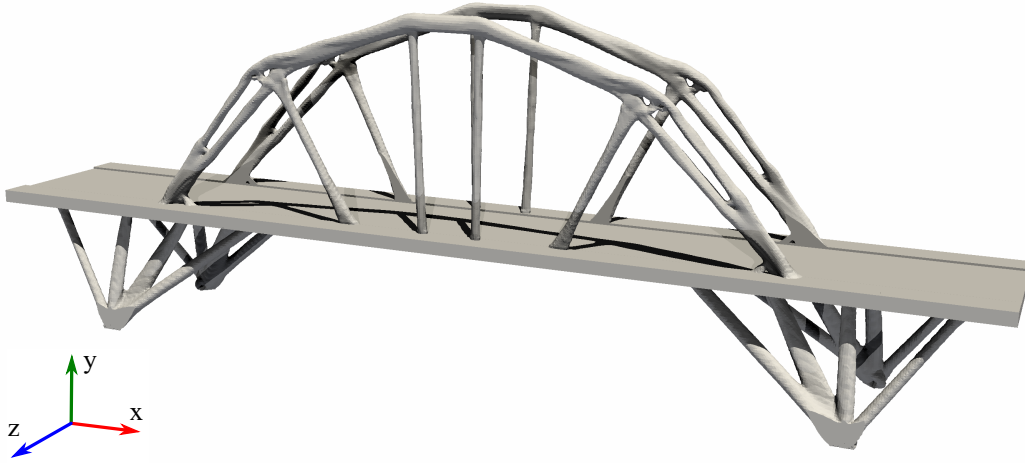
Figure A.15: Bridge. Mean structural compliance optimization. Topology for t=0.94 ( |\Omega^+| = 6\%|\Omega| ).
