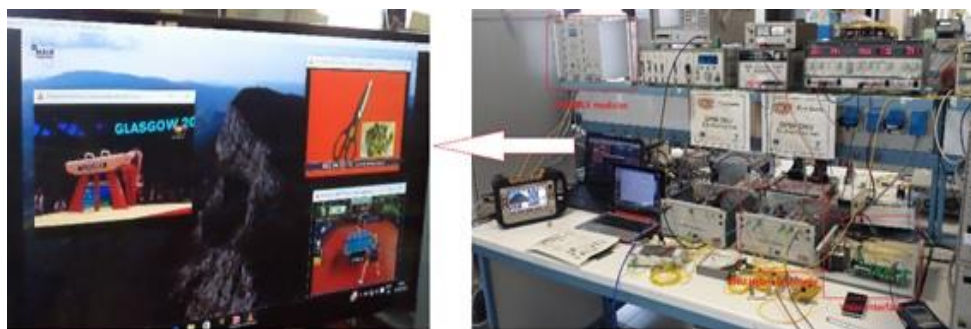
Figure 2.24. (a) Successfully transmitted HD videos during the field-trial demo, (b) Complete heterodyne DPSK ONUs bench.
