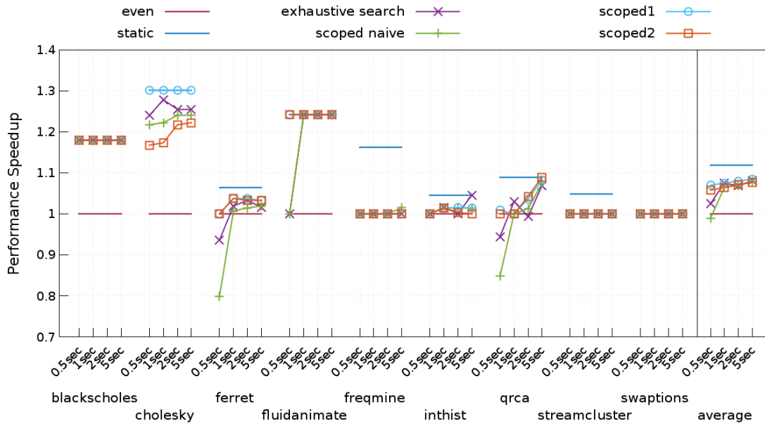
Fig. 5.5 Comparison of best configuration found by exhaustive and scoped online analyses for different monitoring window size, when running under a 80W power constraint. The size of the monitoring window can influence the precision of the analysis.
