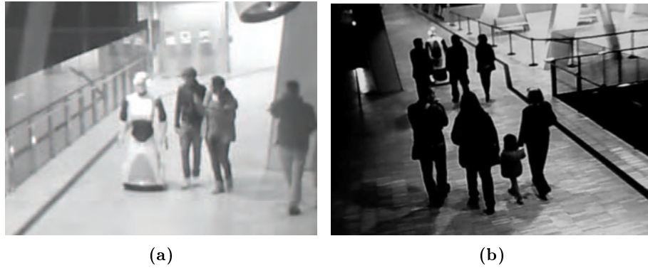
Figure 3.12: follow me spatial arrangement types: (a) walking along with and (b) walking ahead .
