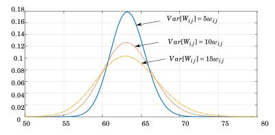
Figure 5.3: The stochastic flow on the AP instance with n = 10 and p = 2 modeled with the Log-normal probability distribution function for different kinds of variance levels k, specifically  $k = \{5, 10, 15\}$ .
