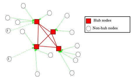
Figure 5.1: Illustrative example of hub network with single assignment and QoS thresholds. In such example, node i can be allocated to different hubs depending on the ammount of stochastic flow that hubs support
