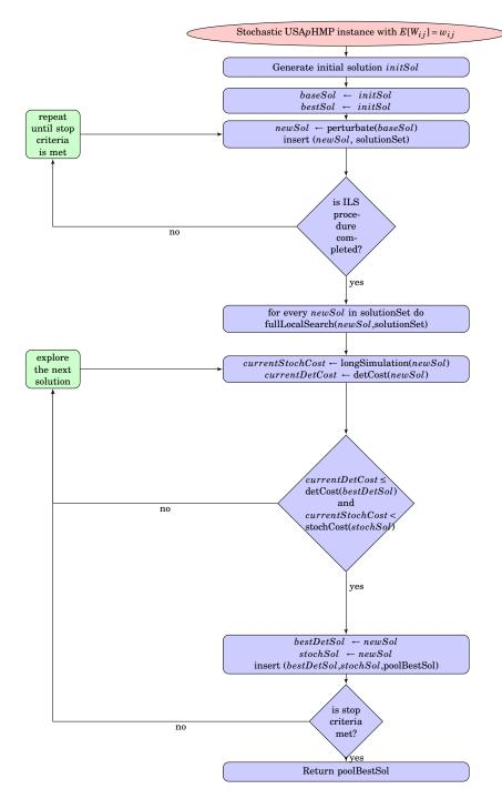
Figure 5.2: Flow-chart diagram of the stochastic USApHMP simheuristic algorithm
