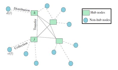
Figure 6.1: Multiple allocation hub-and-spoke network
