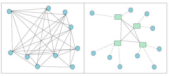
(a) A fully interconnected network with n nodes (b) A multiple-hub network
