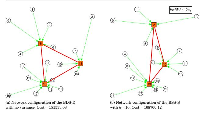
Figure 5.5: Comparison between solutions for the deterministic and stochastic USA*p*HMP, respectively, on a network with 20 nodes and its structure for p = 3.
