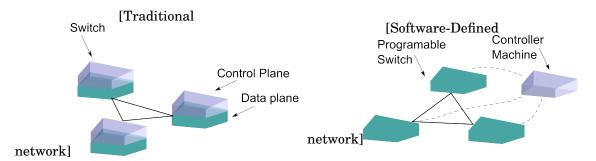
Figure 6.2: Comparison between a traditional network and a software defined network (Maleki et al. 2017)
