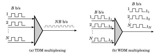
Figure 3.3: Different multiplexing techniques for increasing the transmission capacity on an optical fiber. Both multiplexing techniques take in N data streams, each of B b/s, and multiplex into a single fiber with a total aggregate rate of NB b/s
