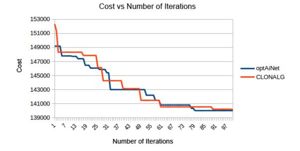
Figure 4.11: Cost of the best solution compared along the iterations by the CLONALG and optAiNet algorithms
