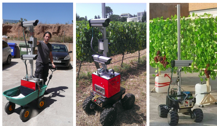
Figure C.16: Vinbot unit phases. Preliminary tested sensor unit on the left, first version in the middle and the fully integrated version on the right.
