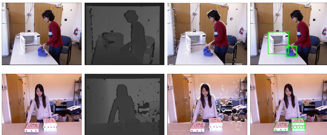
Figure A.5: Multimodal database CAD120 with RGB (most left), Depth map (middle left), 3D map (middle right), object context (most right). Modes for two actions are shown: cleaning and unstacking.
