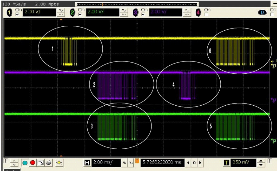
Fig18. Evolution of the wireless communication for three nodes of the network. Node 1 transmit the frame (1). Nodes 2 and 3 receive the frame. As the next hop is node 3, node 2 discards the frame. Finally, node 3 re-transmit the frame to node 2.
