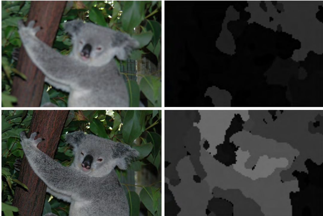
Figure 5.3: Region based sharpness maps. In the top example, the koala is completely out of focus; in the bottom example, the koala is in perfect focus.
