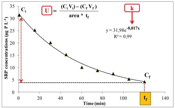
**Figure 1.** Example of dissolved inorganic phosphorus decay in time after controlled spike in response to biotic uptake by river biofilms. Uptake rate coefficient (K, min<sup>-1</sup>) is calculated by fitting negative exponential curve to the data. The phosphate uptake rate (U) was calculated as the mass of phosphorous removed from the water column per unit area per unit time ( $\mu$ g P cm<sup>-2</sup> min<sup>-1</sup>).
