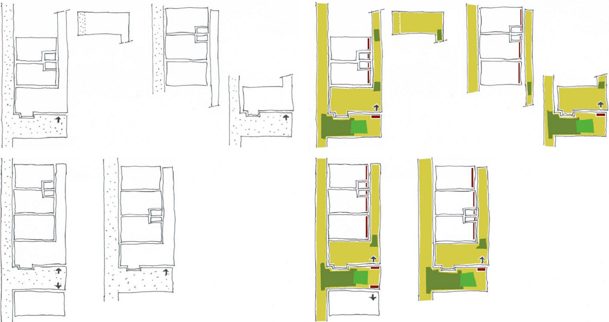
Access Configuration, Territorial Transition, Sequential Gap and Overlap Scenarios in floorplan of different apartment typologies
