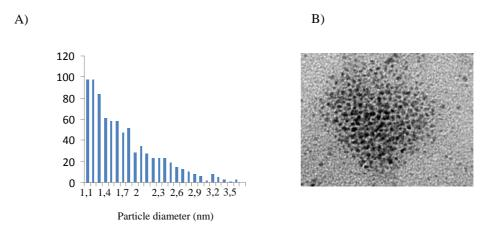
Figure 5.9. "In situ" Pd nanoparticles: A) core size distribution. B) TEM micrograph (x 500000)
