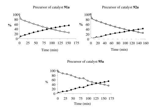
Figure 5.8. Evolution of catalytic diboration of styrene with catalyst precursor 91a, 92a and 95a. Styrene consumption ○, diborane formation ●
