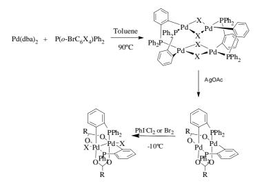
Scheme 5.10. Synthesis of the dinuclear Pd<sub>2</sub><sup>4+</sup>, Pd<sub>2</sub><sup>6+</sup> and tetranuclear Pd<sub>2</sub><sup>4+</sup> complexes
